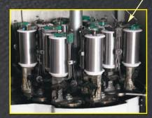
High resistance screen made of a sturdy Aluminium-Magnesium alloy BRAID (AIMg). The braiding process is operated by means of 16 spools braiding machines. Highly effective against low frequency impulsive noises.
